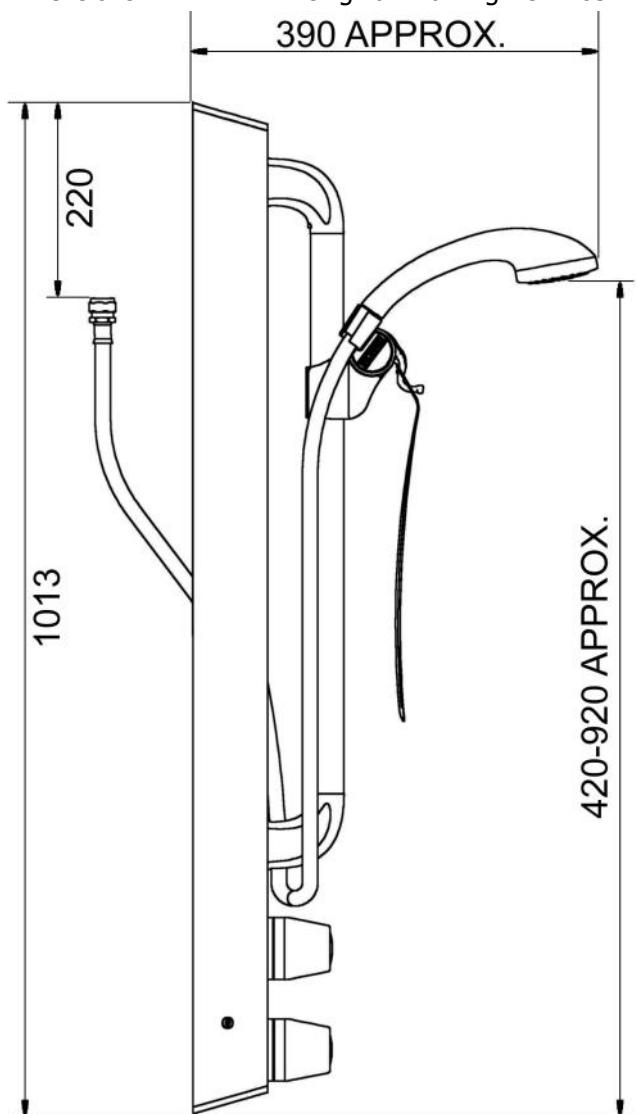
The **T108B** shower panel is pre-plumbed with an integral dual control Type 3 approved thermostatic mixing valve, which features:
