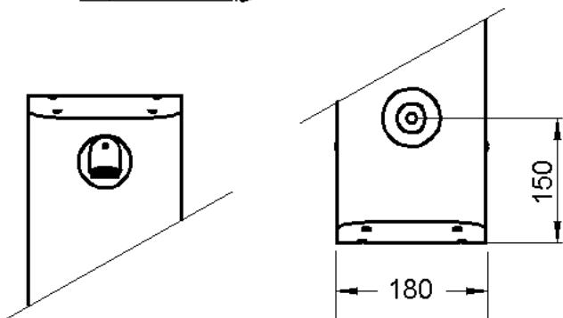
The T109B shower panel is pre-plumbed with an integral Type 3 approved thermostatic mixing valve, which features:
