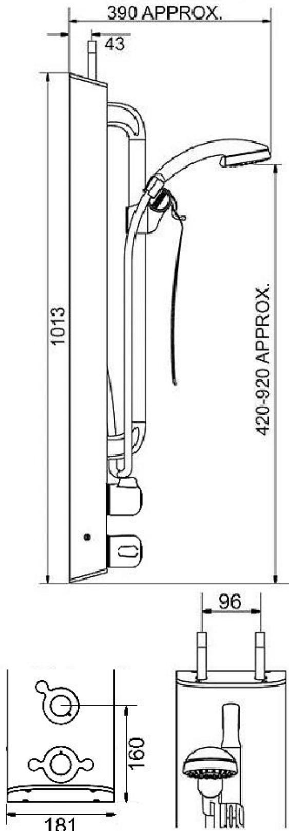
The **T1Y7A2L** shower panel is pre-plumbed with an integral dual control Type 3 approved thermostatic mixing valve, which features:
