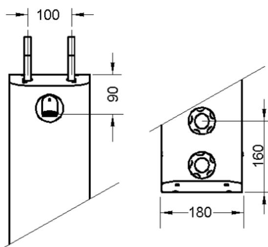
The **T105A** shower panel is pre-plumbed with an integral dual control Type 3 approved thermostatic mixing valve, which features:
