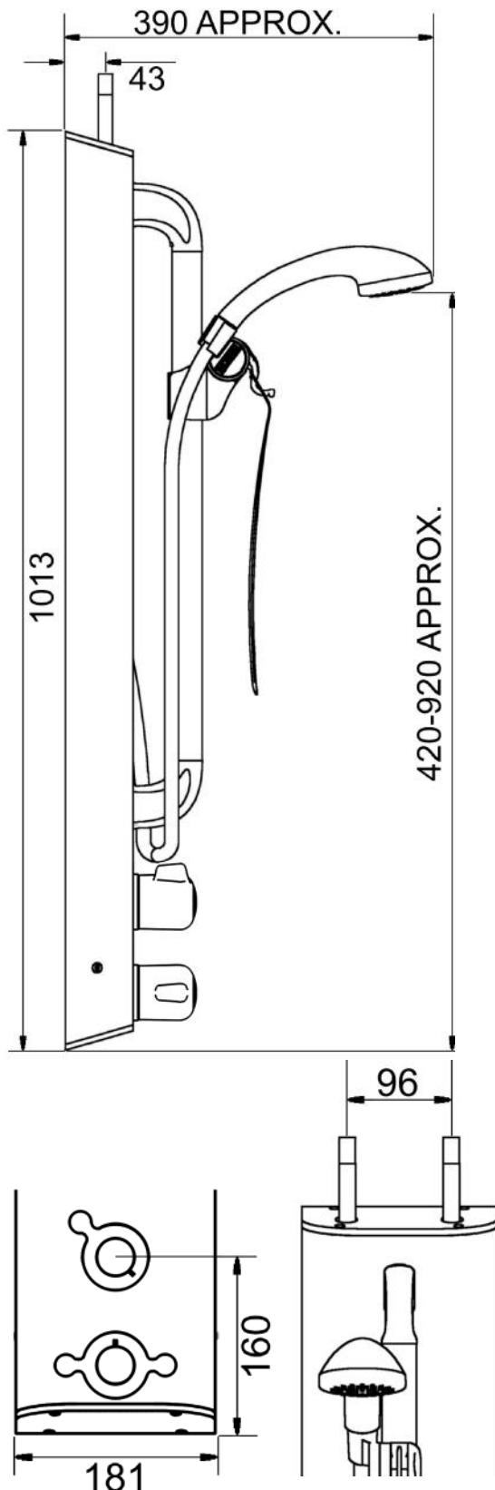
The **T108A2L** shower panel is pre-plumbed with an integral dual control Type 3 approved thermostatic mixing valve, which features:
