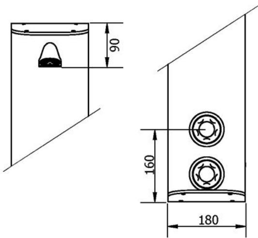
The **T105BLR** shower panel is pre-plumbed with an integral dual control Type 3 approved thermostatic mixing valve, which features:
