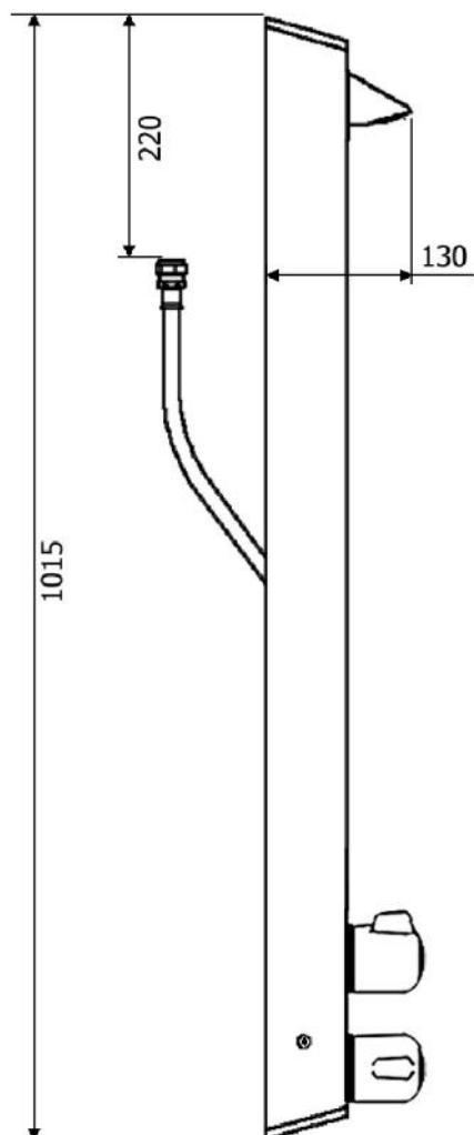
The T105B2L shower panel is pre-plumbed with an integral dual control Type 3 approved thermostatic shower valve, which features:
