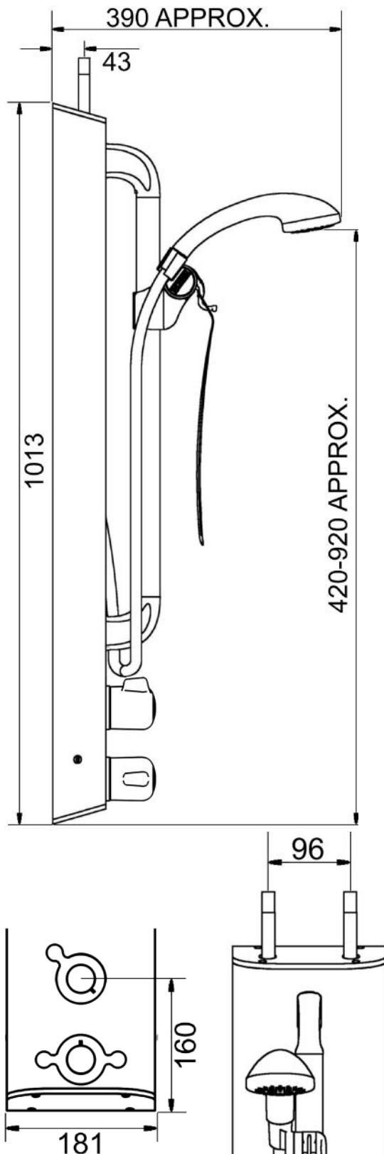
The **T1Y8A2L** shower panel is pre-plumbed with an integral dual control Type 3 approved thermostatic mixing valve, which features:
