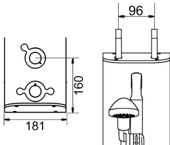
The **T108A2L** shower panel is pre-plumbed with an integral dual control Type 3 approved thermostatic mixing valve, which features:
