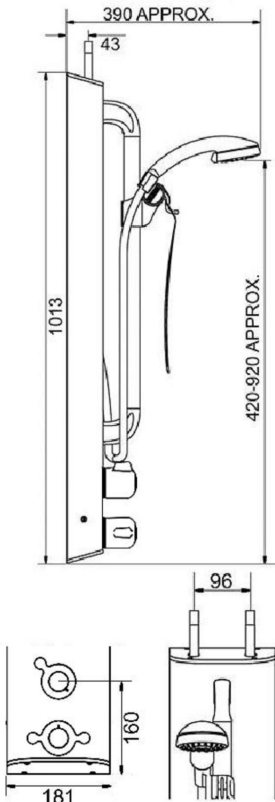
The **T107A2L** shower panel is pre-plumbed with an integral dual control Type 3 approved thermostatic mixing valve, which features:
