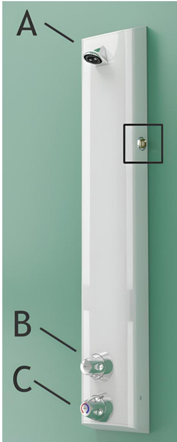
**Unsupervised mode:** The user is able-bodied and does not require supervision during showering. The ligature and vandal resistant outlet (A) is active in this mode. Operation of the shower is by normal means using the ligature resistant flow control (B) to turn on the shower and control (C) to adjust the temperature.
