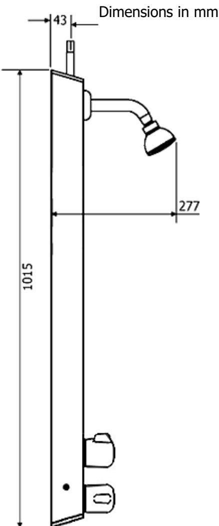
The T106A2L shower panel is pre-plumbed with an integral Type 3 approved thermostatic mixing valve, which features:
