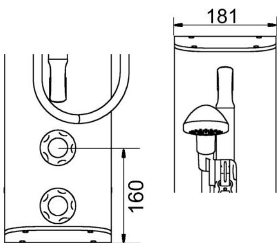
The **T1Y8B** shower panel is pre-plumbed with an integral dual control Type 3 approved thermostatic mixing valve, which features:
