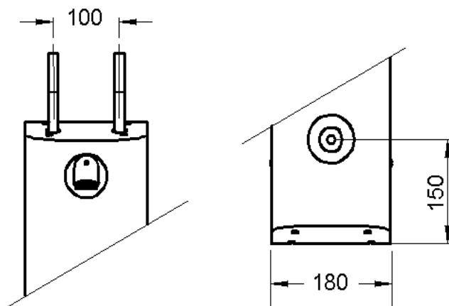
The T109ALR shower panel is pre-plumbed with an integral Type 3 approved thermostatic mixing valve, which features:
