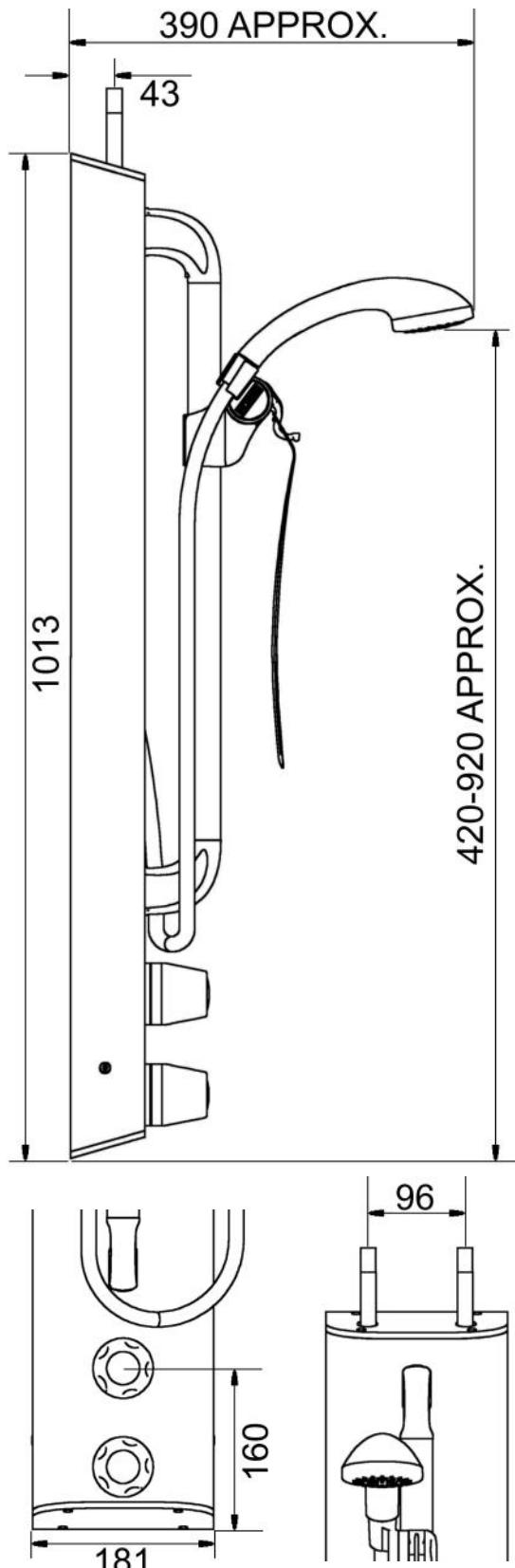
The **T108A** shower panel is pre-plumbed with an integral dual control Type 3 approved thermostatic mixing valve, which features:
