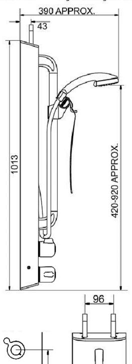
The **T1Y7A2L** shower panel is pre-plumbed with an integral dual control Type 3 approved thermostatic mixing valve, which features:
