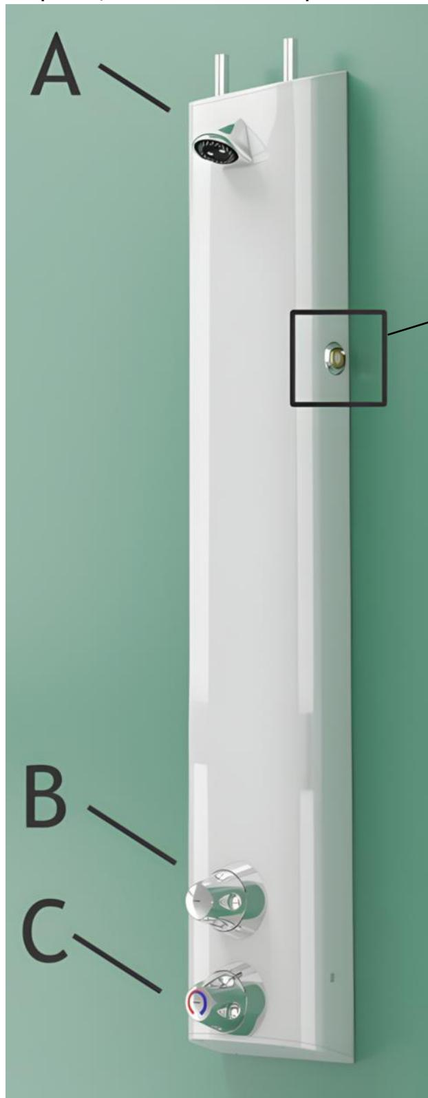
**Unsupervised mode:** The user is able bodied and does not require supervision during showering. The ligature and vandal resistant outlet (A) is active in this mode. Operation of the shower is by normal means using the ligature resistant flow control (B) to turn on the shower and control (C) to adjust the temperature.
