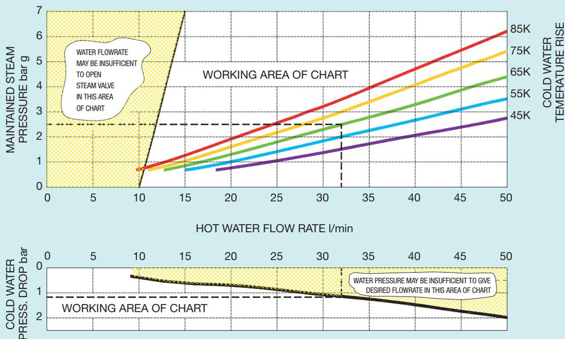
NOTE: THE "MAINTAINED" STEAM PRESSURE REFERS TO PRESSURE WITH THE SUPPLIES RUNNING
