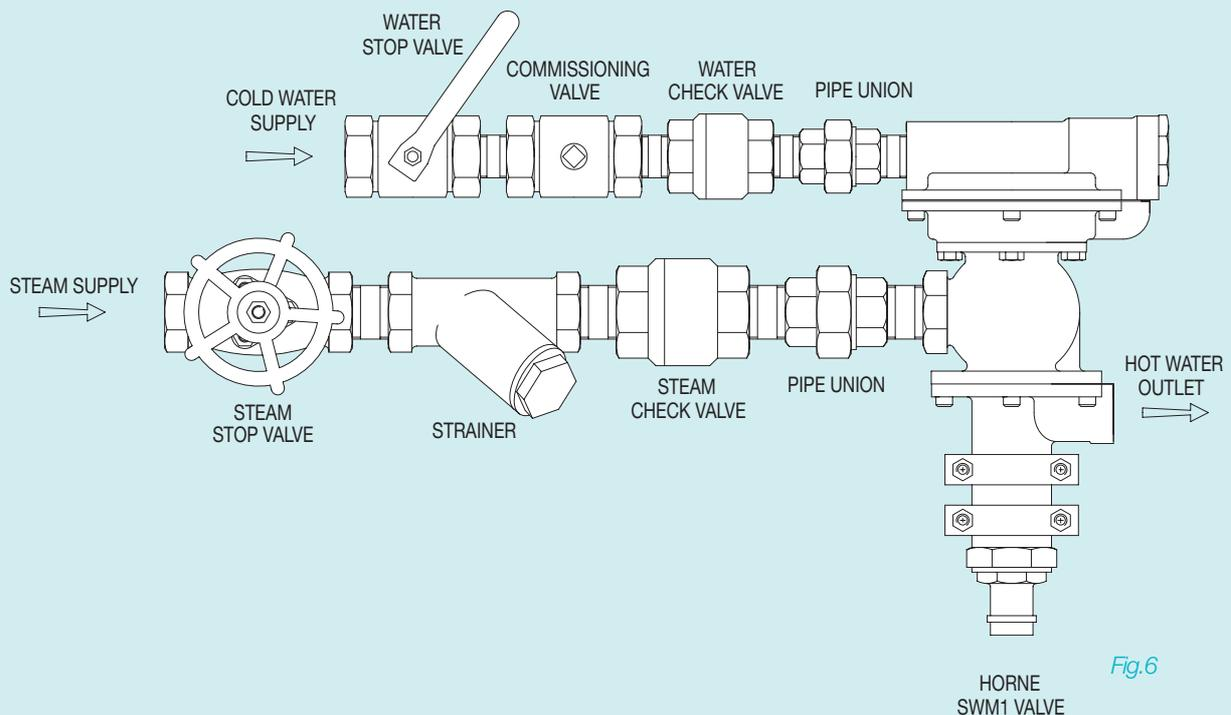
INSTALLATION ARRANGEMENT SHOWING THE NECESSARY COMMISSIONING VALVE, CHECK VALVES, STRAINER, ISOLATING VALVES AND PIPE UNIONS PRE-ASSEMBLED READY FOR INSTALLATION OF THE SWM1 VALVE ON SITE.
