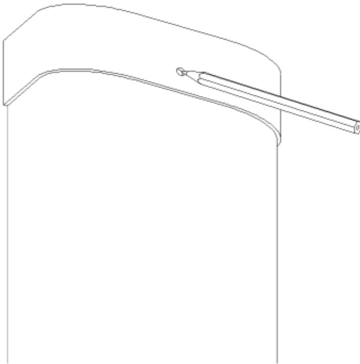
Slide the Pipe Cover down into Place and check for fit. The top of the Pipe Cover should be approx 15mm from the ceiling when pressed firmly into place. Position the Saddle over the top of the Pipe Cover and against the ceiling with the hole in its lower position. Mark through the hole in the Saddle onto the Pipe Cover. See Fig 5.
