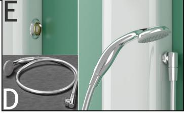
Assisted mode: For able and non ablebodied users who require assistance or supervision during showering. In this mode the carer/supervisor attaches the handset and hose (D) by screwing the hose connector into the ligature and vandal resistant outlet fitting (E) on the side of the panel. Water is <u>automatically</u> diverted to the handset on opening the shower flow control (B). The water temperature (C) is adjusted in the usual way.
