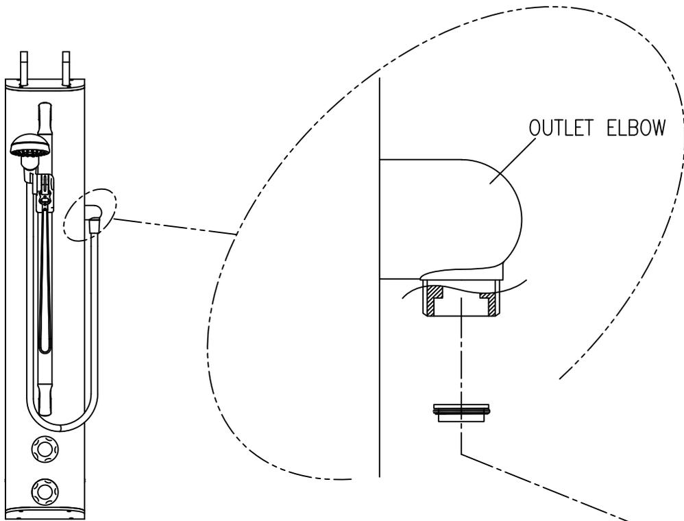
TO REMOVE/REPLACE THE FLOW REGULATOR
