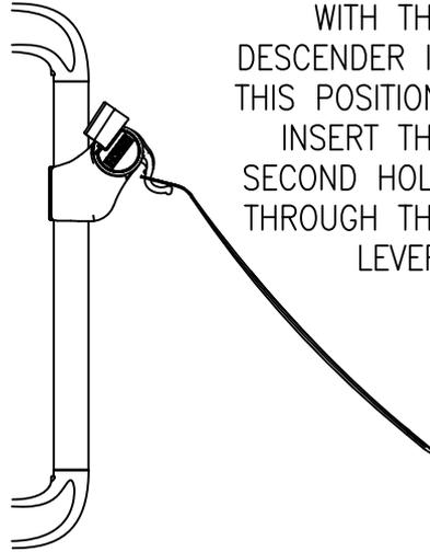
WITH THE DESCENDER IN THIS POSITION, INSERT THE SECOND HOLE THROUGH THE LEVER.
