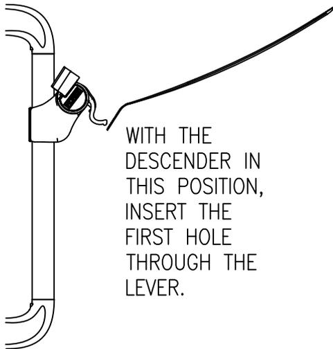
WITH THE DESCENDER IN THIS POSITION, INSERT THE FIRST HOLE THROUGH THE LEVER.
