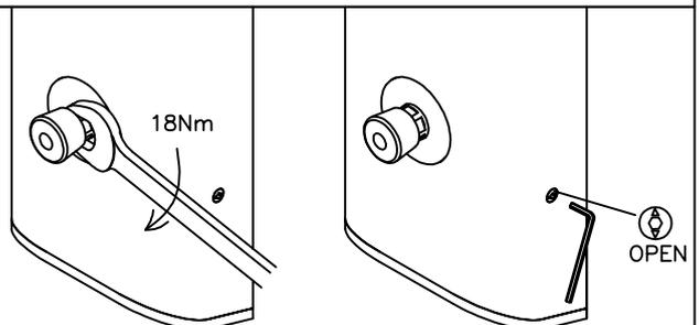
PUT THE CARTRIDGE BACK INTO THE SHOWER PANEL. TIGHTEN DOWN TO 18Nm. OPEN THE HOT AND COLD SUPPLIES AT THE SERVICING VALVES. THE INDICATOR ARROWS ON THE SERVICING VALVES WILL POINT UP AND DOWN WHEN THE SUPPLIES ARE OPEN. PUSH THE BUTTON TO PURGE THE AIR AND THEN VERIFY THE PERFORMANCE OF THE CARTRIDGE.
