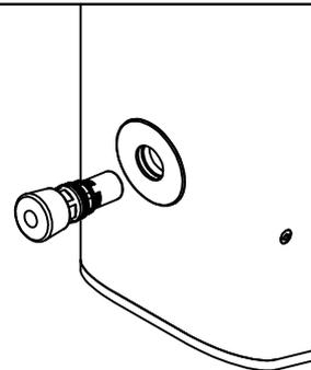
REMOVE THE TIMED FLOW CONTROL CARTRIDGE. BE CAREFUL NOT TO DROP THIS PRECISION PIECE OF EQUIPMENT. DO NOT PUT IT DOWN ANYWHERE WHERE IT COULD BECOME CONTAMINATED WITH DIRT OR DUST, NOR WHERE IT COULD BE STOOD ON.
