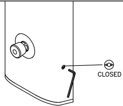
USE A HEX KEY TO ISOLATE THE HOT AND COLD WATER SUPPLIES AT THE LOW LEVEL SERVICING VALVES. THE INDICATOR ARROWS ON THE SERVICING VALVES WILL POINT TO THE FRONT AND THE BACK OF THE PANEL WHEN THE SUPPLIES ARE ISOLATED.
