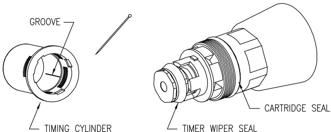
IF THE TFC CARTRIDGE BECOMES JAMMED (WON'T MOVE OUT TO CLOSED POSITION), REMOVE THE CARTRIDGE IN ACCORDANCE WITH STEPS 2-4, THEN PULL THE TIMING CYLINDER FROM THE CARTRIDGE ASSEMBLY. CLEAN OUT THE GROOVE INSIDE THE TIMING CYLINDER BY GENTLY RUNNING THE SHARP END OF A PIN UP AND DOWN THE GROOVE. A SMALL AMOUNT OF DEBRIS SHOULD BE DISLODGED BY THIS ACTION. THE TIMING CYLINDER MAY BE RINSED UNDER CLEAN RUNNING WATER - ABRASIVES SHOULD NOT BE USED.
