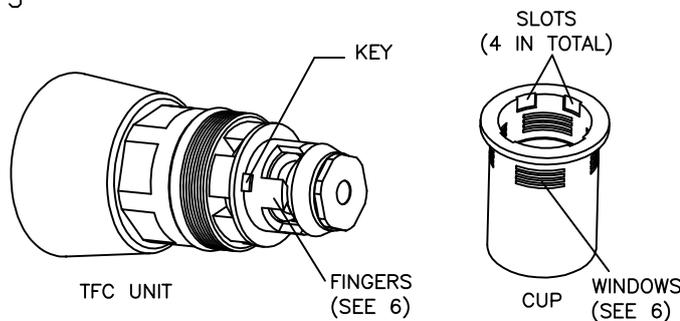
THE TFC UNIT HAS A KEY WHICH FITS INTO ONE OF 4 SLOTS IN THE CUP. THERE ARE THEREFORE 4 ORIENTATIONS OF THE TFC IN THE CUP. EACH OF THESE GENERATES A DIFFERENT FLOWRATE AND FLOW DURATION.
