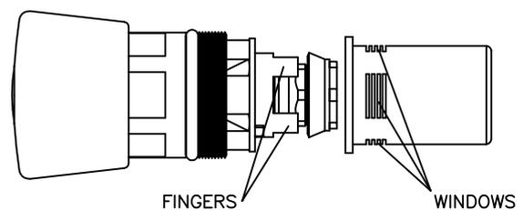
THE TFC UNIT HAS FINGERS WHICH BLANK OFF "WINDOWS" IN THE CUP WHEN ASSEMBLED. THE 4 ORIENTATIONS CORRESPOND TO 4 DIFFERENT DEGREES OF BLANKING. SECTION 7 SHOWS CLOSE-UP VIEWS OF THE WINDOWS AND EXPLAINS THE SIGNIFICANCE OF EACH ORIENTATION
