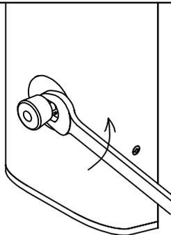
PRESS THE PUSHBUTTON TO RELEASE ANY TRAPPED PRESSURE. USING A SLIM JAW 24mm SPANNER ON THE HEX UNDER THE PUSHBUTTON, UNSCREW THE TIMED FLOW CONTROL CARTRIDGE.
