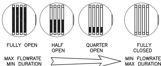
THE TFC UNIT HAS FINGERS WHICH COVER THE "WINDOWS" IN THE SIDE WALL OF THE CUP. SELECT THE MOST APPROPRIATE COMBINATION AS ABOVE, AND PUSH THE CUP ONTO THE CARTRIDGE.
