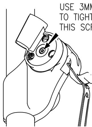
USE 3MM HEX KEY TO TIGHTEN OR LOOSEN THIS SCREW.
