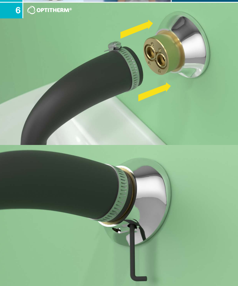
Flush pipework after spigot installation
