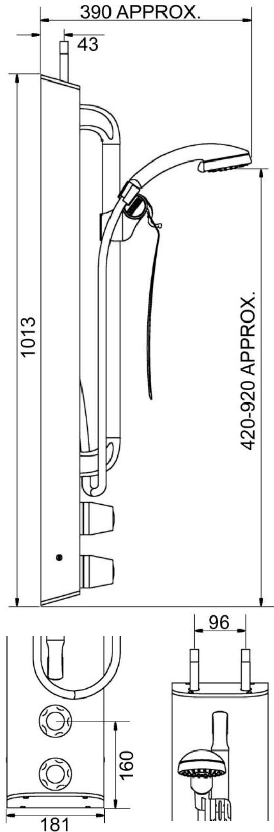
The **T107A** shower panel is pre-plumbed with an integral dual control Type 3 approved thermostatic mixing valve, which features:
